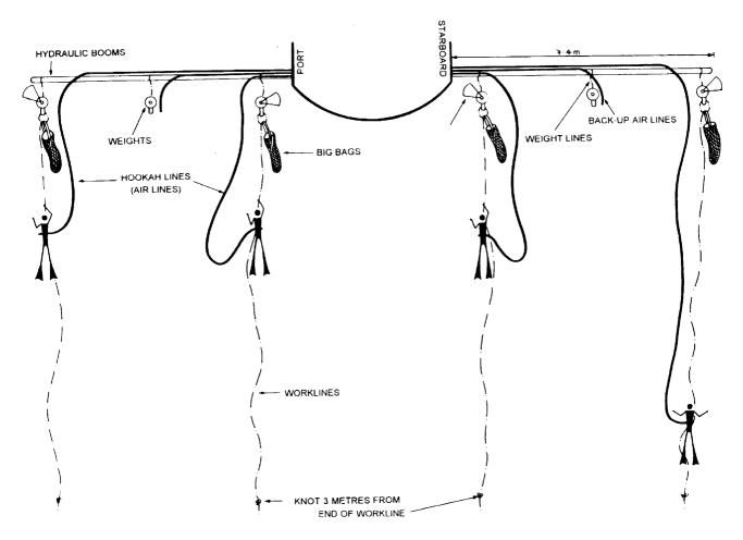
Figure 3. Plan view of pearl fishing operation
