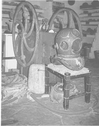
Figure 2. A pump, helmet, hose and breastweight: relics of sponge diving in Symi a hundred years ago.
