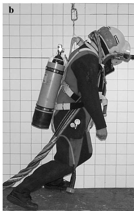
Figure 2 The diver may be lifted into the bell with the hoist attached either anteriorly (a) or posteriorly (b). This is often assisted by partial flooding of the bell to help float the diver through the hatch.
