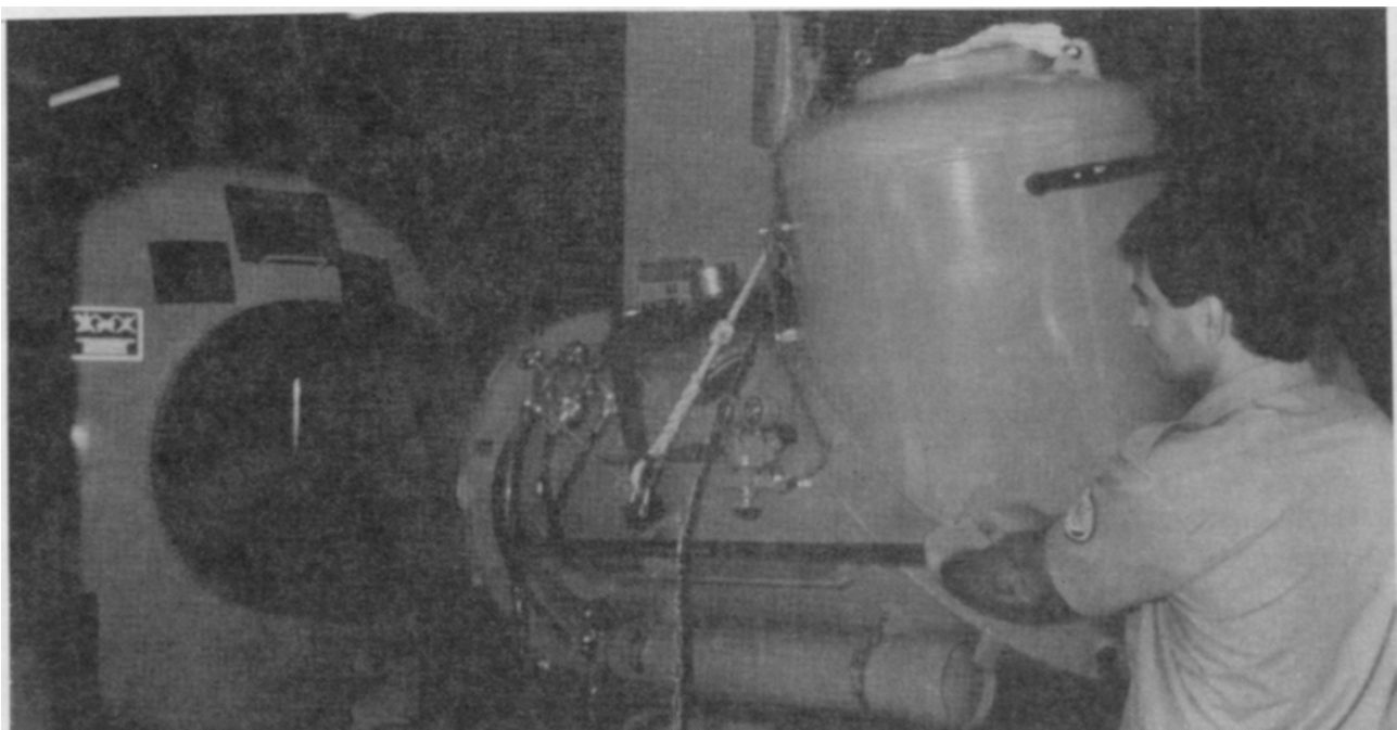
Figure 1. The Townsville Recompression Chamber (RCC), (showing the transfer-under-pressure flange for DuoCom attachment, generously donated by the Utah Foundation of Australia.)
