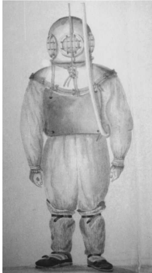
Figure 5. 1840, the new “tight” dress had a loose flange, designed by George Edwards, added to a Deane helmet manufactured by Augustus Siebe.
