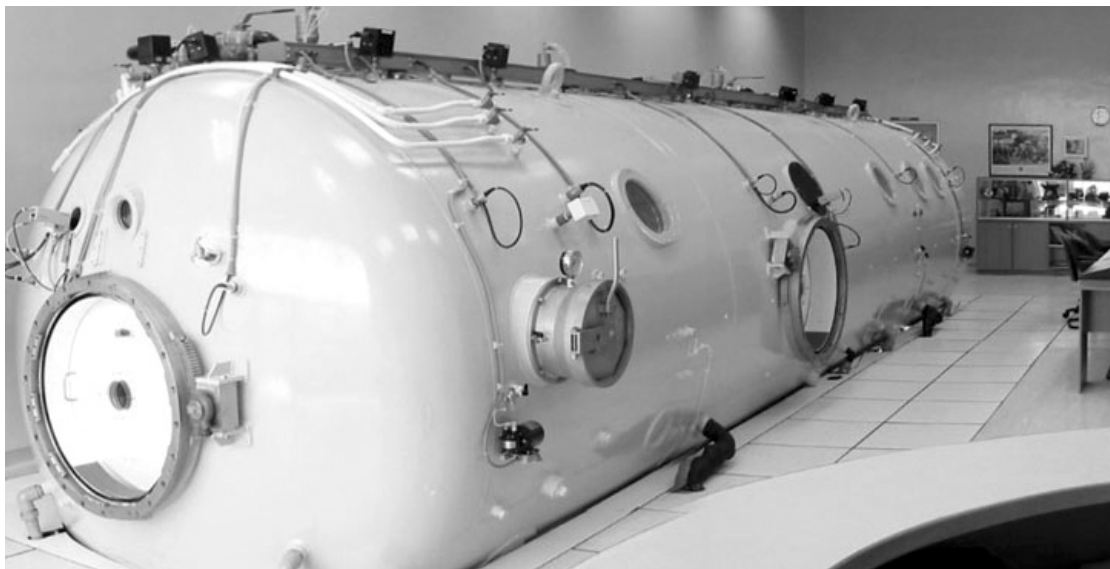
Figure 1 The three-compartment multiplace recompression chamber in the Institute of Underwater and Hyperbaric Medicine (IUHM) at Armed Forces Hospital in Lumut (source: IUHM)
