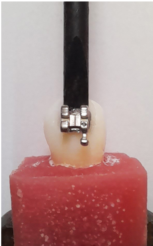
Figure 1 Shear bond strength testing configuration
