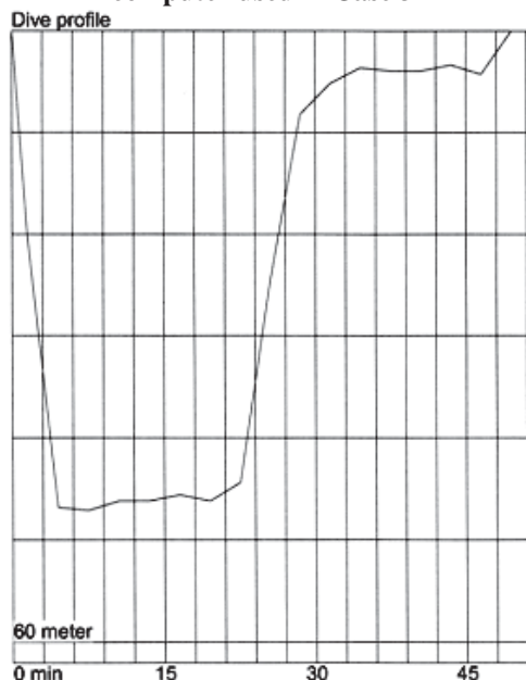
Figure 3 Download of the incident dive from the Buddy Nexus computer used in Case 3
