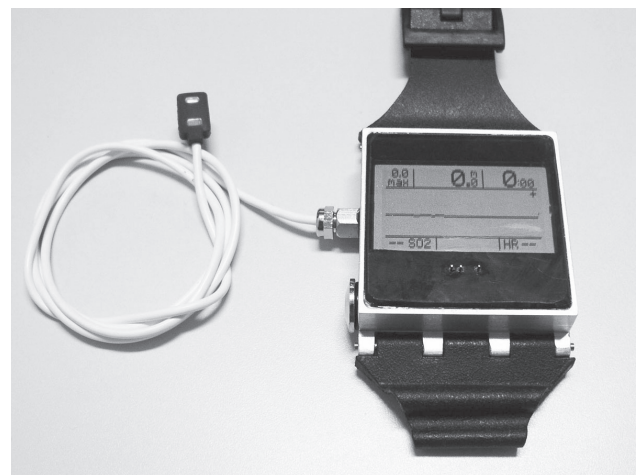
Figure 3 The prototype wrist-mounted apnea diving computer
