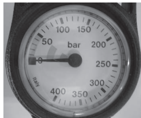
Figure 1 Submersible pressure gauge with lowest 50 bar coloured coded (usually red)
