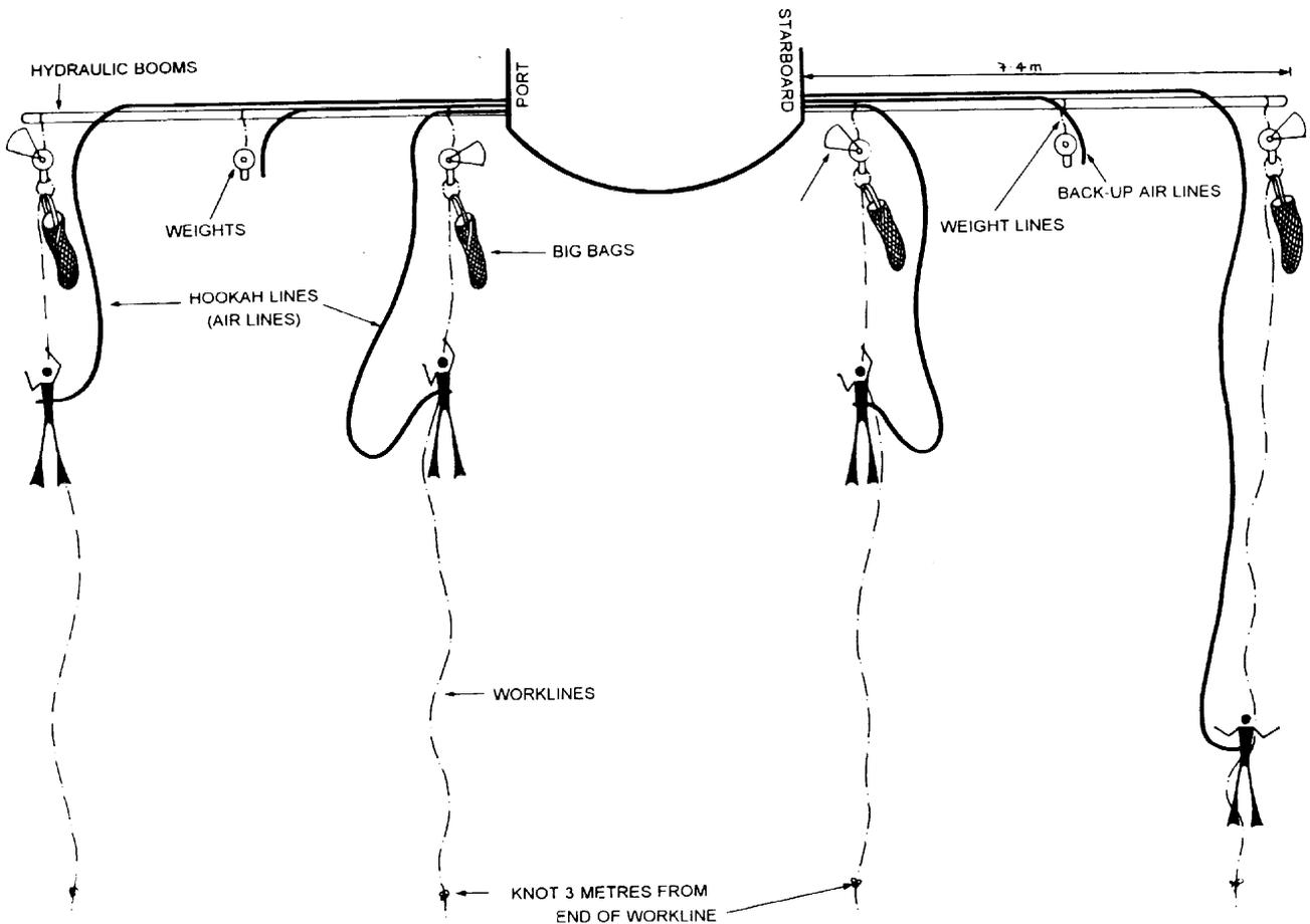
**Figure 3.** Plan view of pearl fishing operation
