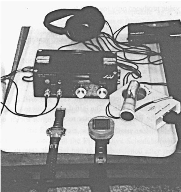
**Figure 2.** Equipment for Doppler monitoring. Showing chest probe, Suunto depth recorder, Hyperaqualand depth/time recording watch, tape recorder and ear phones.
