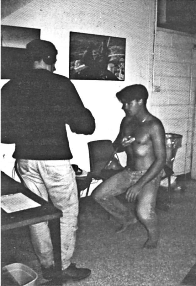
**Figure 3.** Doppler equipment being used. The volunteer is doing knees bends as controlled exercise to provoke bubbling.
