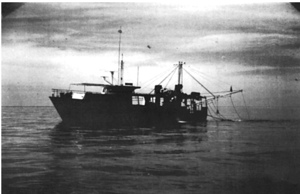
*A modern pearling vessel out of Broome showing outriggers, lines and hoses*
