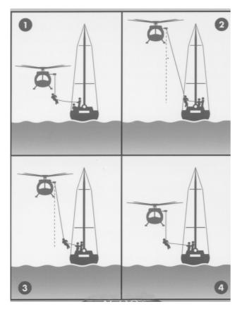
Once the line has been taken by the deck crew, the helicopter will move away from the vessel to prepare the winchman for lowering to the deck. At this time the deck crew must pay out the Hi-line. After winching out the winchman, the helicopter will climb to a safe height over the masts and obstructions whilst lowering the winchman to keep him level with the transfer area. The deck crew should take up the slack in the Hi-line so that the winchman does not swing.
