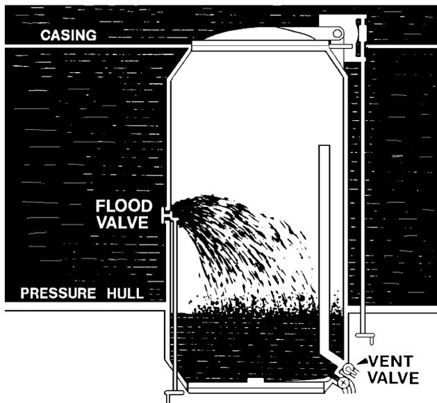
**Figure 4.** Single-man escape tower, for use by escaper with Hood Inflation System, shown when flooding up and venting into the submarine, with no change in pressure in the escape tower, before the phase of rapid pressurisation of the remaining air lock. [from Ref 23]
