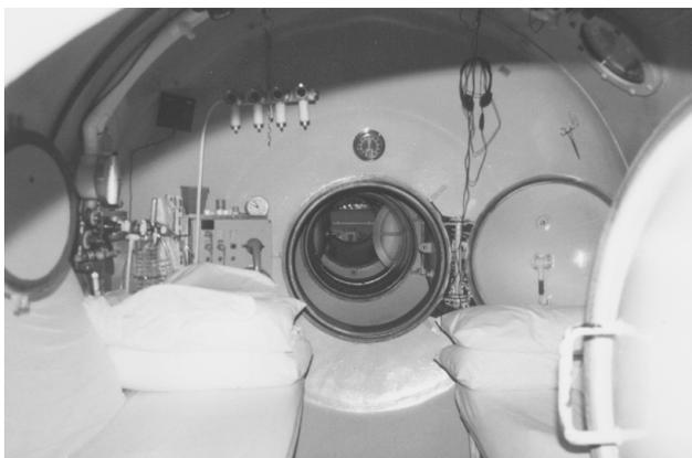
**Figure 2.** Looking through the Vidor chamber with its 800 mm doors, only just wide enough for a stretcher to be passed through, into its second compartment and then on into the other compartments. On the left can be seen the oxygen supplies for the patients.
