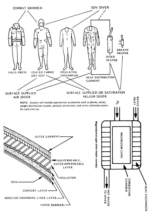
Because dry suits derive much of their insulation from gas trapped between the diver and suit, each suit was tested with nitrogen and helium as the suit gas.
