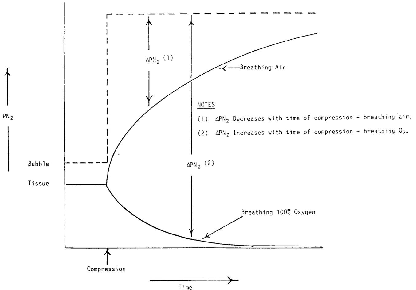
FIGURE 2. Effect of compression on the  $PN_2$  gradient from a bubble using air and 100%  $O_2$ .
