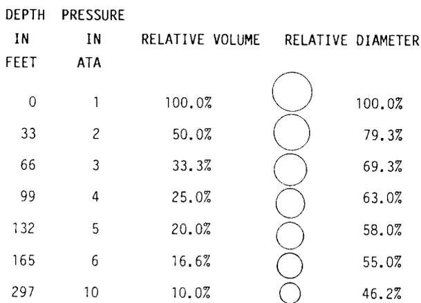
FIGURE 1. Bubble volume and diameter changes with pressure changes.<sup>3</sup>
