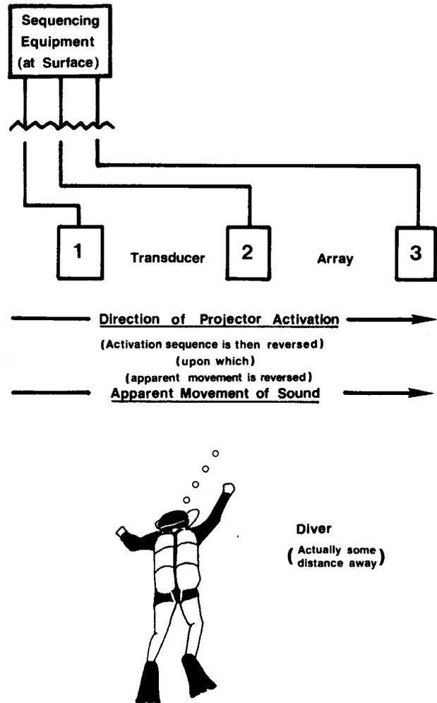
**Figure 3.** This drawing portrays the procedure by which the diver navigates. The sound attracts him to the target by first moving from left to right (from J-11-1 to J-11-3) and then from right to left (J-11-3 to J-11-1) and so on.
