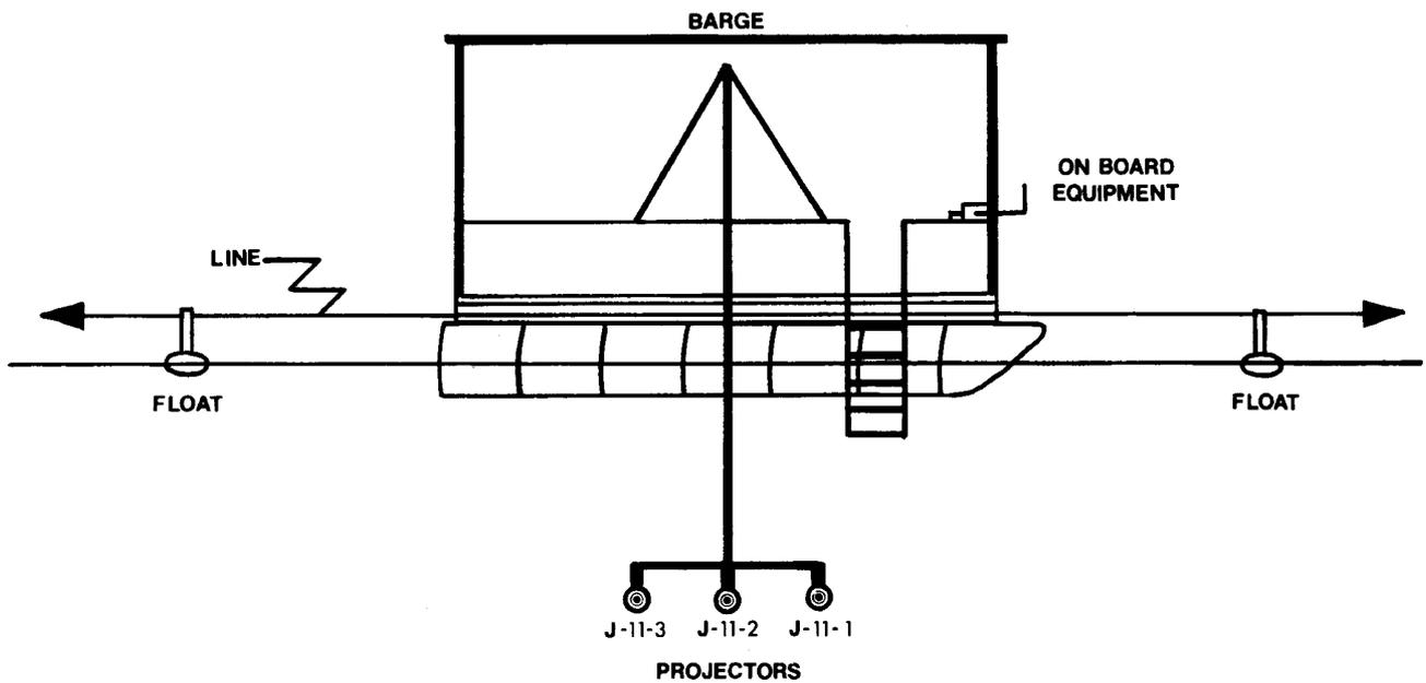
Figure 1. Schematic diagram of the barge, the transducer array and the plane (float to float) also included as part of the target.
