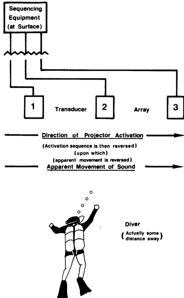
**Figure 3.** This drawing portrays the procedure by which the diver navigates. The sound attracts him to the target by first moving from left to right (from J-11-1 to J-11-3) and then from right to left (J-11-3 to J-11-1) and so on.
