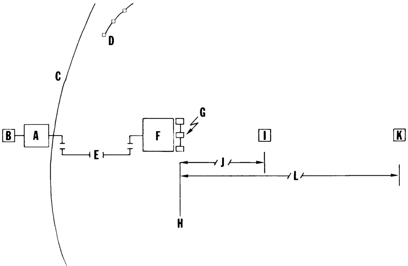
Figure 2. A schematic drawing of the range used in many of the UAPP experiments. A is the equipment van, B a generator and C is the shore. Line E carries the signal to the staging equipment on barge E. The J-11 s are placed 7m under the barge (see also Figure 1) and "hits" are counted when the diver passes line H (between the floats anyway). The range is depicted by L and the starting point by K (I and J refer to other experiments).
