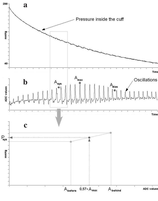
(user definable), it is deflated at about 2–3 mmHg per second. During deflation, an algorithm detects all positive peaks of the oscillations inside the cuff. These peaks are stored in a two-dimensional array together with the pressure inside the cuff. Additionally every peak is shown on the display, in combination with the actual pressure inside the cuff in mmHg.
