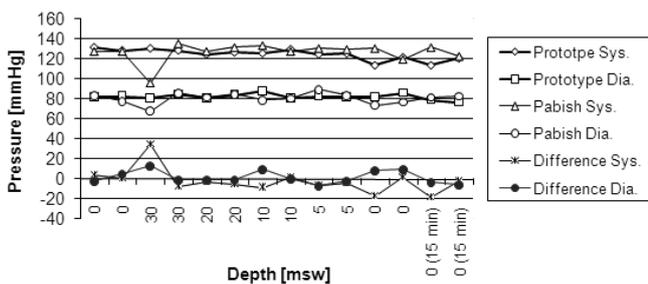
prototype. This is likely caused by the environmental noise in the hyperbaric chamber, which makes it difficult to detect the Korotkoff sounds accurately.
