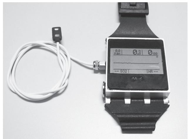
silicone gel (SilGel 612, Wacker Chemie AG). Further, this measure allows installation of the digital pressure sensor directly on the electronic board, as the ambient pressure is transduced via the soft silicone gel to the membrane of the pressure sensor. Only the battery is housed in a water- and pressure-proof compartment.
